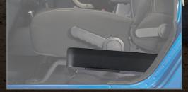
The subwoofer plug & play system mounts to the driver's seat factory assembly for improved bass/mid-bass performance, even when the top is off.
